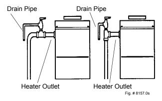
**NOTE:** To avoid water damage or scalding due to valve operation, drain pipe must be connected to valve outlet and run to a safe place of discharge. Drain pipe must be the same size as the valve discharge connection throughout its entire length and must pitch downward from the valve. No shut-off valve shall be installed between the relief valve and the drain line. Valve lever should be tripped at least once a year to ensure that waterways are clear.
